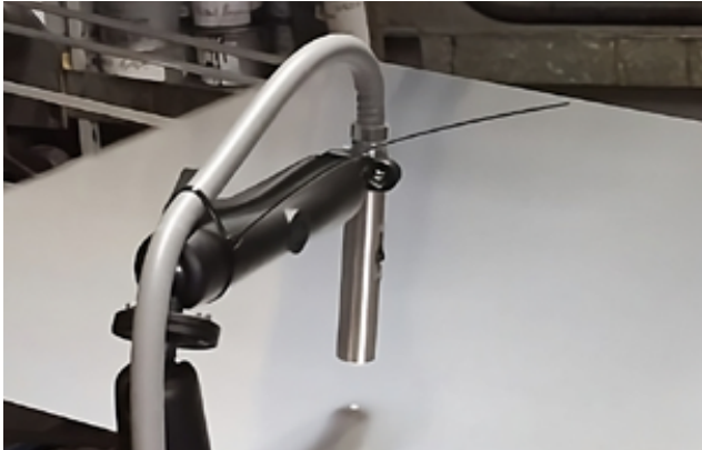
▲ Periodic in-process measurements via magnetic arm with ruggedized probe.
