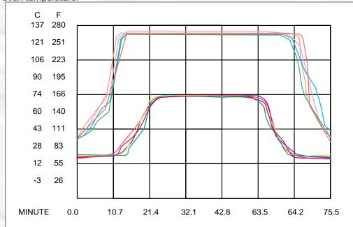
**Taiyo** Circuit Automation Temperature Profile: Rapid ramp-up allows full utilization of heated zone to maximize productivity. Temperature uniformity unmatched by competitive ovens: ± 1°C at tack-dry temperatures.
